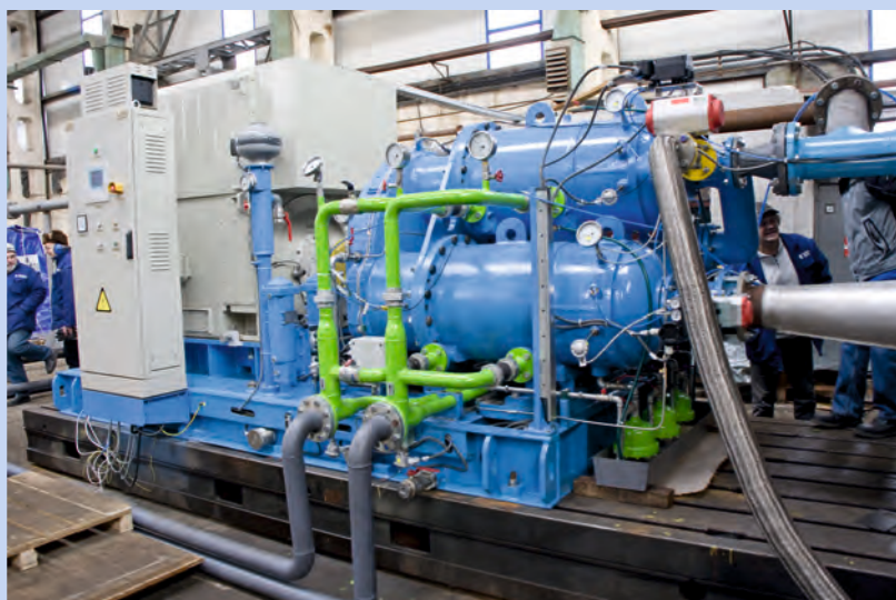
Compressor CCAE 9-125 (intercooled) on the test rig.
