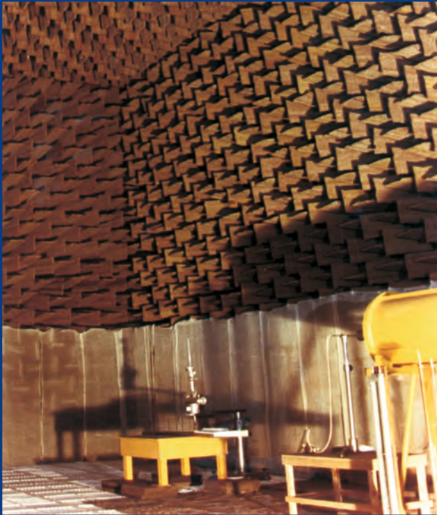
Acoustic tests - Anechoic chamber (1,200 m 3 ).
